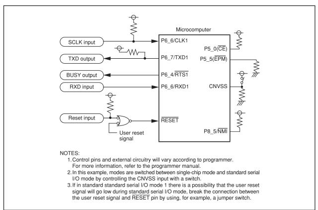
Figure 20.15 Circuit Application in Standard Serial I/O Mode 1
